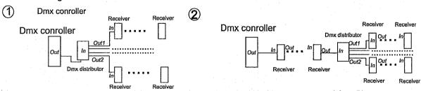
Receiver can not more than 32 units on one out channel Use one terminator on the last receiver. Push on the push button. Nothing on link out put. Receiver can not more than 31 units before Dmx distributor Receiver can not more than 32 units on one out channel Use one terminator on the last receiver.
