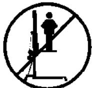
**3.1** - The TE-086 is a machine designed to elevate loads upwards in a vertical direction, It should NEVER be used as a platform to elevate people.
