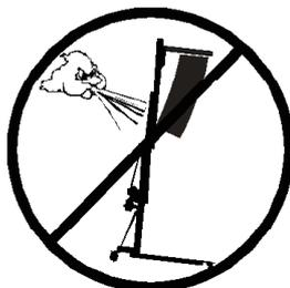
**3.7** - If there is a possibility of strong winds or gusts, place the lift on the ground firmly and secure it with the use of straps. NEVER attach a strap to a vehicle or any other object that can possibly be moved.
