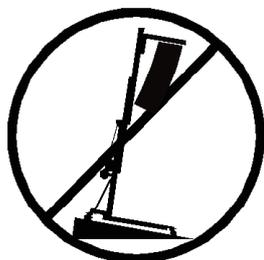
**3.2** - Only place the lift on hard, flat surfaces always checking that it is in a vertical position by using the bubble level indicator (**L**) found on the base section. Adjust the leg stabilizers (**Q**) by turning the handles (**H**) to level if necessary. NEVER use wedges or other foreign objects to balance the lift.
