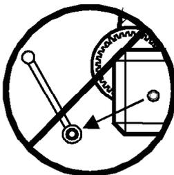
**3.16** - NEVER take apart the crank of the winch when the lift is carrying a load or extended.
