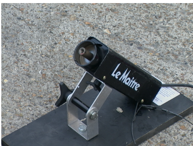
The solenoid unit mounted on a board
