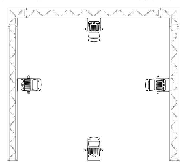
The Spectra Spot 40 can be operated in a number of mounting positions as shown in the diagram above, hanging upside-down from the ceiling or truss, mounting sideways on truss or stood upright on a flat level surface. Always use a safety wire as an extra safety precaution to prevent damage/injury in the event a clamp fails (see the next page for clamp installation). Never use the carry handles for secondary attachments.
