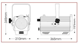
Stylish, compact and high efficiency RGBW led power source, fresnel luminaire featuring 120mm diameter Fresnel lens and DMX/RDM controllable for 16 bit dimming and infinite colour beams.
