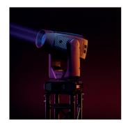
The Furion H402 Hybrid is a highly adaptable moving head that combines beam, spot and wash effects in a single light fixture that is capable of illuminating the grandest of stages. Equipped with a 420 W discharge lamp, its optical prowess allows smooth transitions between a narrow 0.6° beam and a wide 50.7° wash for ultimate flexibility. Its beam diffuser ensures even light distribution without hotspots, making it perfect for concerts, theatrical productions, live events and more.
