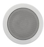
The Apart EN-CM6T6 is a 6.5" built-in ceiling speaker made of powder coated steel (RAL 9010 equivalent), equipped with a high efficiency full range speaker and a multi tap 100 volt transformer, all certified according EN 54-24. The unit is equipped with a ceramic speaker line connector block, thermal fuse and a metal fire dome.
