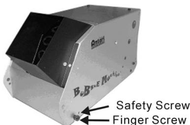
To help avoid accidental exposure to dangerous live AC mains voltage, two safety screws are fitted that require a screwdriver to remove. Once these are removed, the finger screws can be undone by hand (see photo above).
