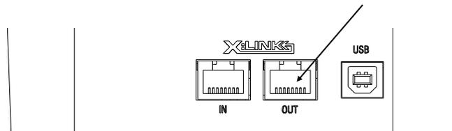
Connect the RJ45 cable to the X:LINK socket of the XONE:43C mixer.
