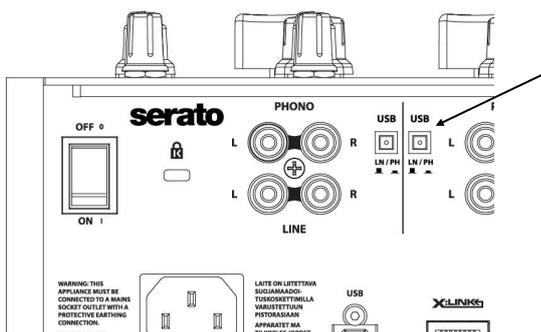
On the channel input that has the turntable or CD Media player connected, select the appropriate USB select switch for Phono or Line.
